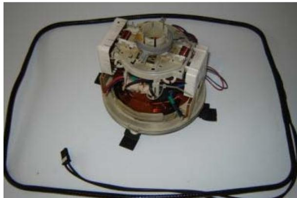
9 & 10 CRT Yoke (centre) & Degaussing coils
