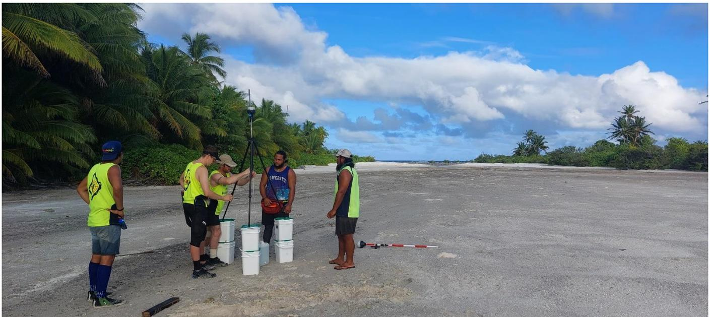
Above: Setting up the RTK base unit to broadcast on Cooks Motu
