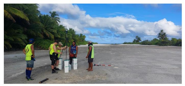
Above: Setting up the RTK base unit to broadcast on Cooks Motu
